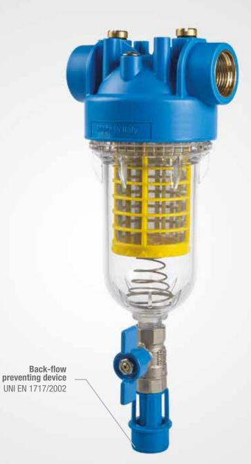
Max working pressure: 8,3 bar (120 psi). Min working pressure: 1,2 bar (17.4 psi). Max working temperature: 45°C (113°F). **Materials:** Reinforced PP, PET, CW 617 N brass nickel plated, stainless steel.
