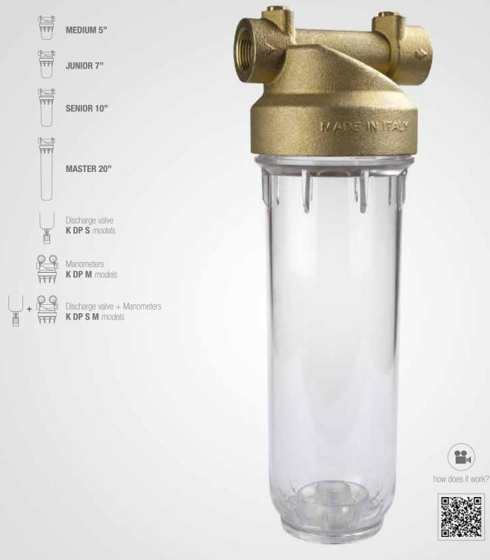
Max working pressure: 10 bar (145 psi). Max working temperature: 45°C (113°F). Materials: Brass CB 753 S, PET. Accessories:
