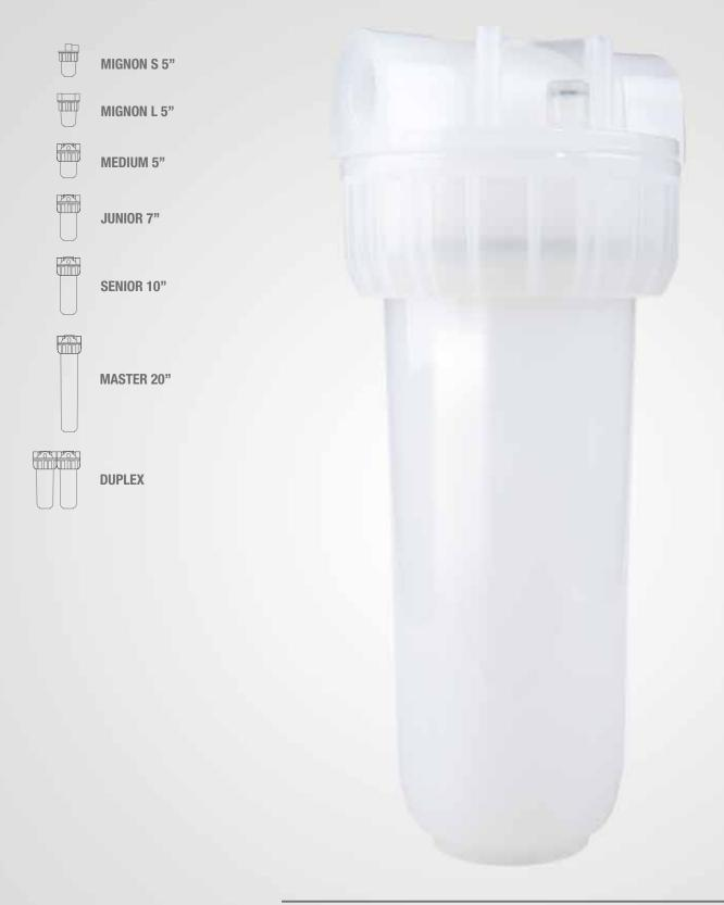
Max working pressure: 3 bar (43 psi) water with non neutral pH 8 bar (116 psi) water with neutral (7) pH. Max working temperature: 35°C (95°F). pH: 2 - 10. Materials: PP. Accessories:
